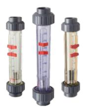
These flowmeters operate according to the variable area principle, where a float is suspended in upward flowing media in a tapered plastic tube. The vertical position of the float within the metering tube depends on the flowrate of the media. The metering tube is graduated in suitable flow units and the reading is taken in correspondence with the top edge of the float. Versions for liquids and gases are available, providing accurate and cost-effective measurement with scales in I/h and Nm3/h
